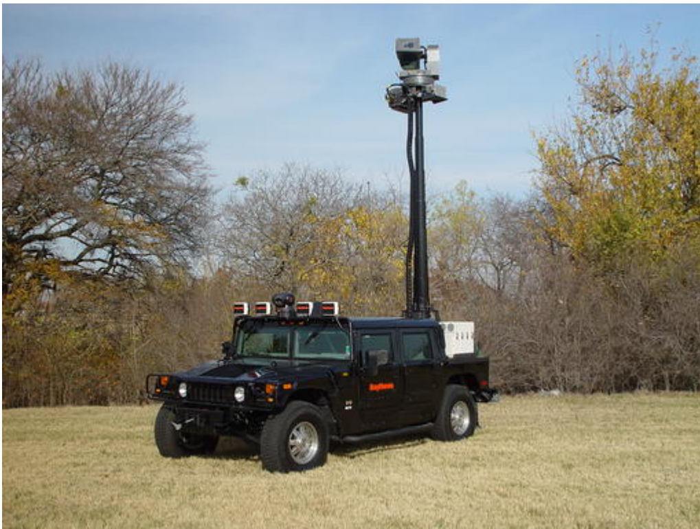
Figure 1. RSTA-MEP system mounted on a Hummer with mast extended. The sensors are at the top of the mast; the embedded systems are in white boxes on the back. The crewstation computer is inside the vehicle.
